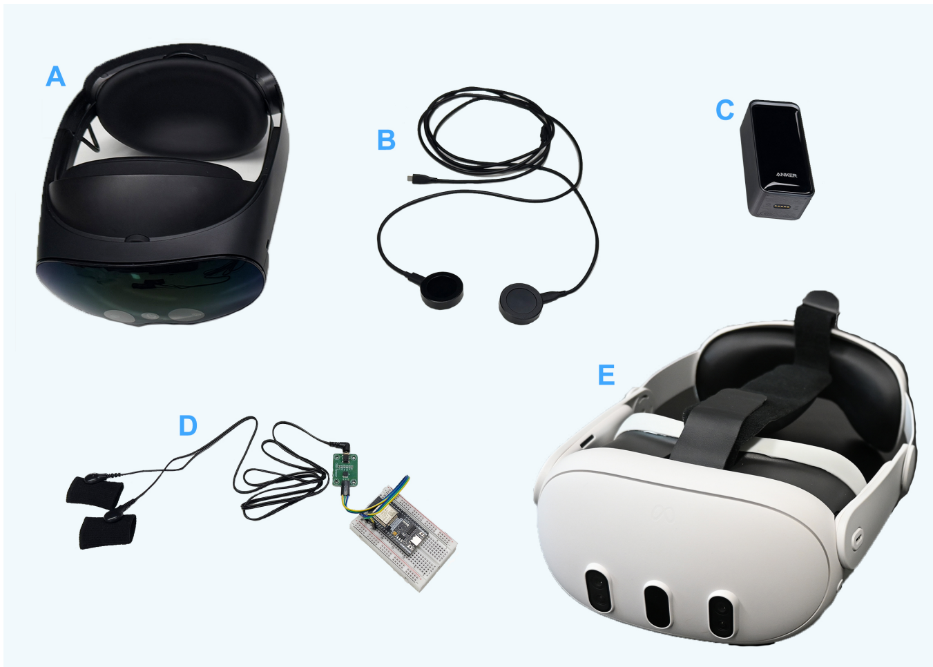
Figure 3: Components of the E.A.T. system: A) a Meta Quest Pro headset used for XR food augmentation and external expressive displays; B) circular external LCD displays with connecting cables for visualizing pupil movement and physiological arousal; C) a portable power bank used to supply external components; D) a GSR sensor with ESP 32 and wiring; E) a Meta Quest 3 headset used for XR food augmentation without external displays.
